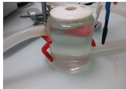
5% of hydrochloric acid solution before coupon immersion.
